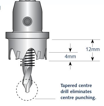
From measurements Ø 16 mm to 30.0 mm, the hole saw is made of one piece. From Ø 31.0 mm, we use specially hardened tool holders to compensate for the torsional power in case of heavy operation, which avoids early shearing off of the tool holder shank. As such, its construction is incomparable with any other design.
